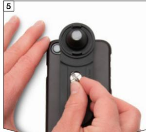
**5** Loosen the screw slightly.
